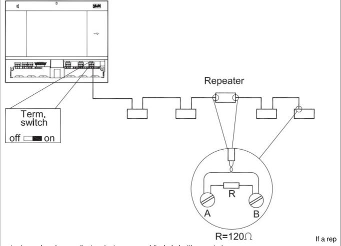
eater is used, make sure the terminators are used (included with repeater). Use the included 120 Ohm terminator on last device.
