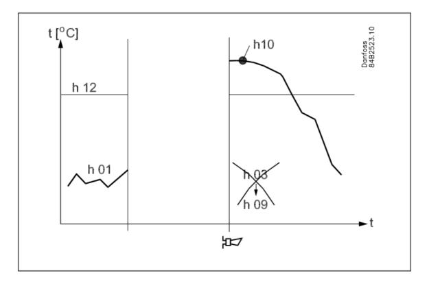
The readout of the various values in the HACCP function can take place with a long push on the middle button. The readouts are, as follows:
