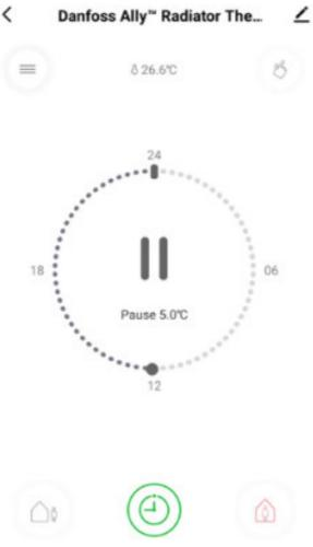
When Danfoss Ally™ is turned down to Min level manually, a notification banner is shown, and the center icon switches to 'Pause'.
