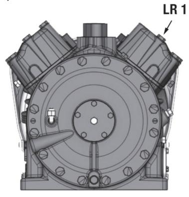
Delivery condition 1 (from the factory): Cylinder cover prepared for capacity regulator.
