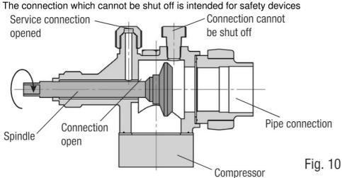
After activating the spindle, generally fit the spindle protection cap again and tighten with 14-16 Nm. This serves as a second sealing feature during operation.
