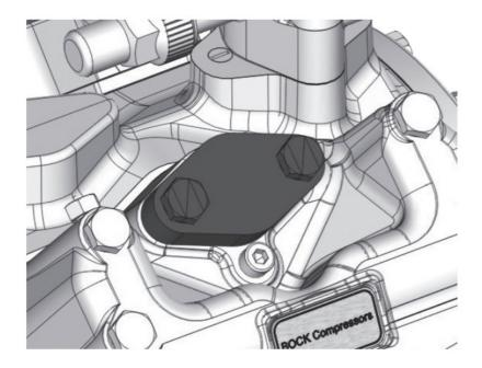
Before commissioning, the blind flange with screws must be removed and replaced by the new set capacity regulator with O-ring joints and screws. Observe position and construction of the capacity regulator.
