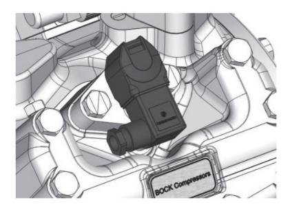
WARNING Several capacity regulators cannot switch at the same time during compressor operation! Otherwise the sudden change in load can damage the compressor! Comply with the switching interval of 60 s.
