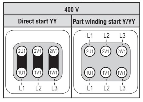
**ATTENTION** Failure to do this results in opposed rotary fields and results in damage to the motor. After the motor starts up via partial winding 1, partial winding 2 must be switched on after a maximum delay of one second. Failure to comply can adversely affect the service life of the motor.
