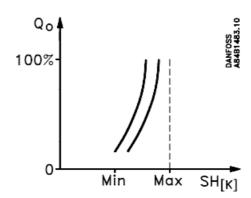
Regulation is here based on the evaporator's load by means of MSS search (MSS = lowest permissible superheat).
