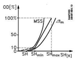
The reference follows a defined curve. This curve is defined by three values: the closing value, the min. value and the max. value. These three values must be selected in such a way that the curve is situated between the MSS curve and the curve for average temperature difference  $\Delta$ Tm (temperature difference between media temperature and evaporating temperature. Setting example = 4, 6 and 10 K).
