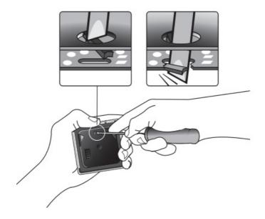
If you break the small plastic seal on the back of the display module, e.g. using a screwdriver, it will be possible to set the maximum floor temperature up to 45°C. Furthermore, it will be possible to use only a room sensor. However, this option is not recommendable due to an increased risk of overheating the floor.
