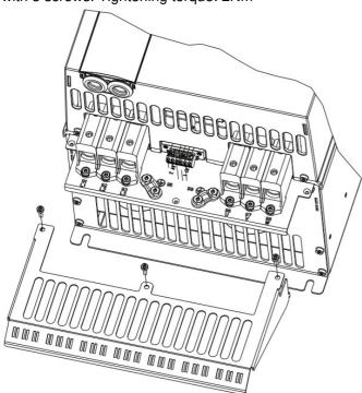
**Step: 2**VLT HVAC Basic Drive mounted with decoupling plate
