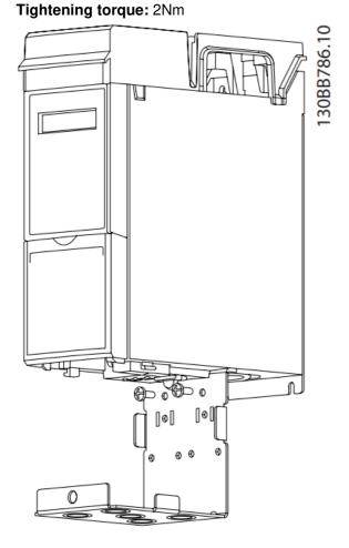
**Step 3**Fit bottom cover onto frequency converter and tighten a M4 X 10 screw.
