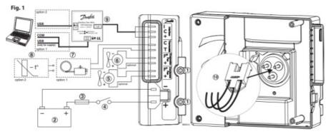
Connect the terminal plug from the electronic unit to the compressor terminal (10). Mount the electronic unit on the compressor and fix it with the two screws (1).
