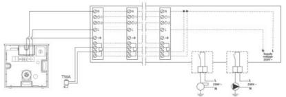
Connection of more thermal actuators to one thermostat (bridging).
