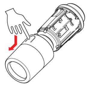
3. Press firmly on the tab and unscrew the thermostat from the adapter
