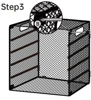
Align screw B with the screw hole and tighten screw B.
