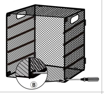
Align screw B with the screw hole and tighten screw B.
