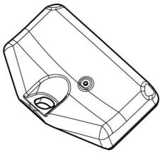
The sensor is used in conjunction with the valve stem, and together they are mounted on the vehicle's wheel hub for the purpose of monitoring tire pressure.
