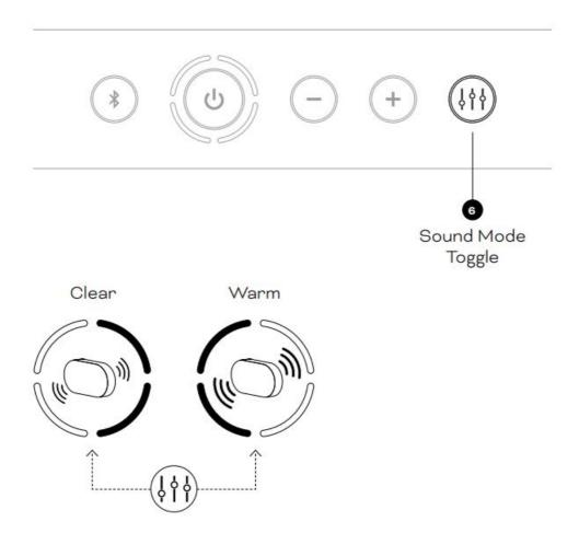
If two KATCH G2 speakers are connected to each other in TWS mode, the sound mode must be adjusted individually on both units.
