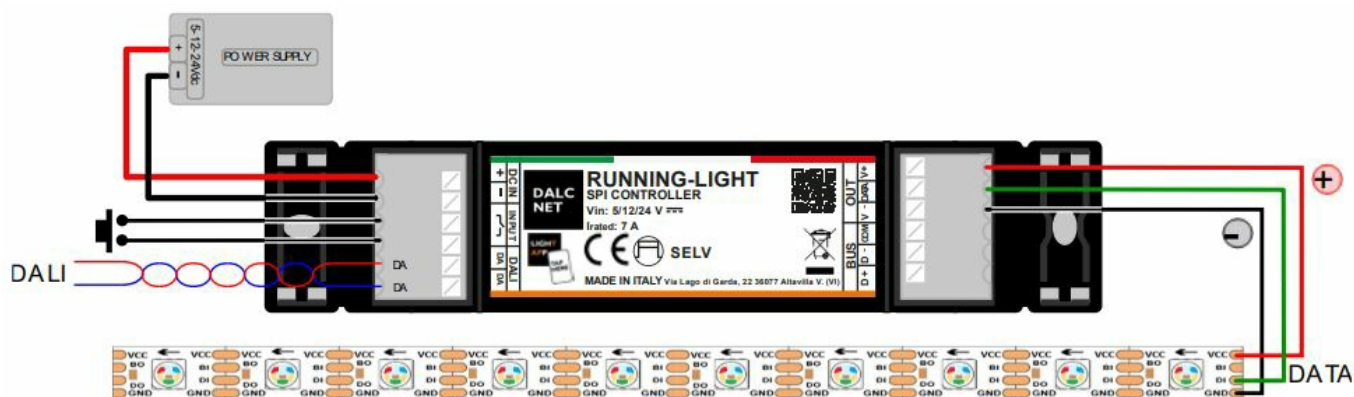
Figure 2: Connection diagram for Digital LED loads
