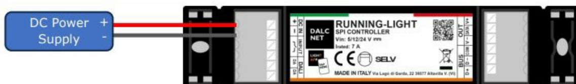
Figure 10: Power Supply Connection Diagram
