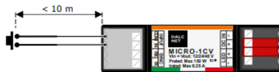
Figure 3: Push-button wiring diagram recommended for Short Distances
