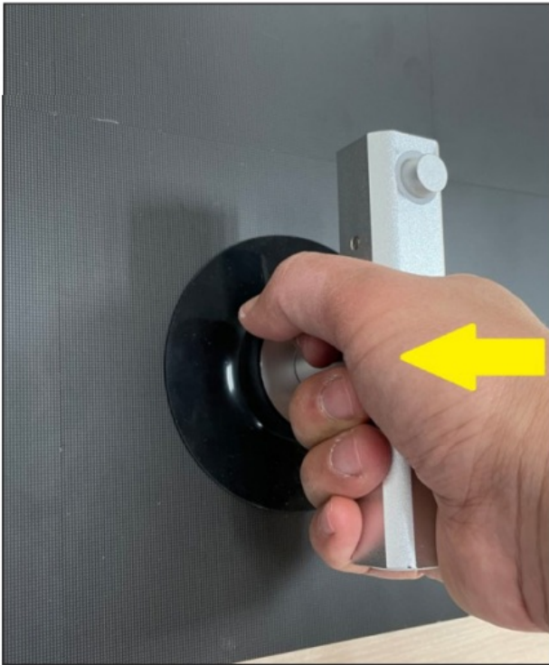
Figure 3: Push Removal Tool onto the Module
