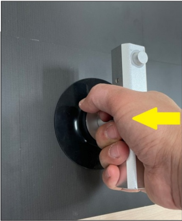
Figure 3: Push Removal Tool onto the Module
