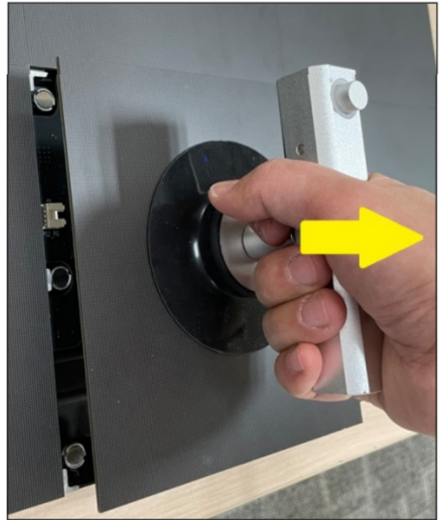
Figure 4: Pull the Module out by Holding the Removal Tool
