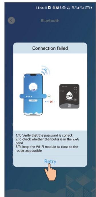
Fig.30-2 Can't connect to the wifi interface
