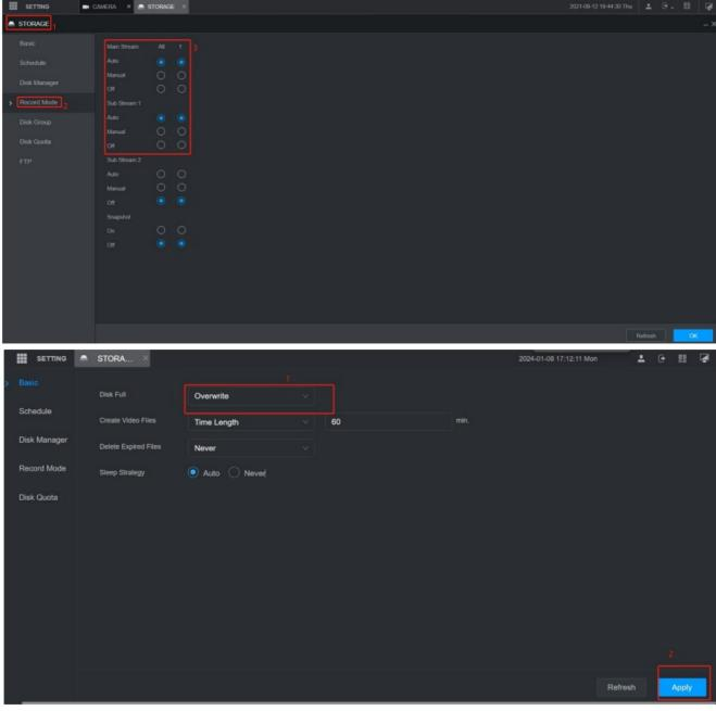
4. open the overwrite, When the hard disk recording is full, the system will automatically overwrite the oldest video
