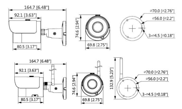
**Installing the Camera Installation Methods**
