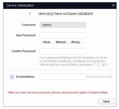
**Step 7** Set and confirm the password of the devices, then enter a valid email address, and then click Next. The final setting interface is displayed.
