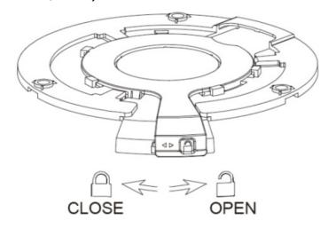
• When the mounting plate is at the "open" state, you can install, adjust, or remove the camera; and when it is at the "close" state, the camera is fixed.
