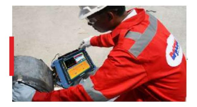
**Phased array technology** is the ability to electronically modify acoustic wave characteristics such as beam angle, and focusing. Probe modifications are performed by introducing time shifts in the signals sent to and received from individual elements of a probe array. Any ultrasonic techniques for flaw detection and sizing can be applied using phased-array probes. This technology has made major advancements with respect to weld scanning, corrosion scanning, and difficult to inspect materials.
