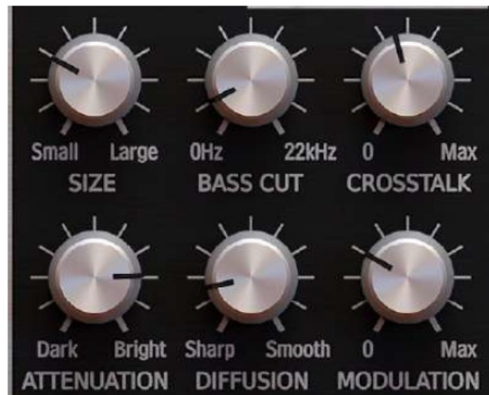
Section controlling Late reflections' tail
