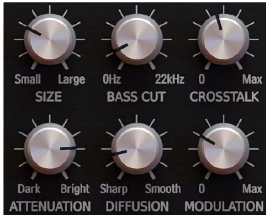
Section controlling Early reflections' tail
