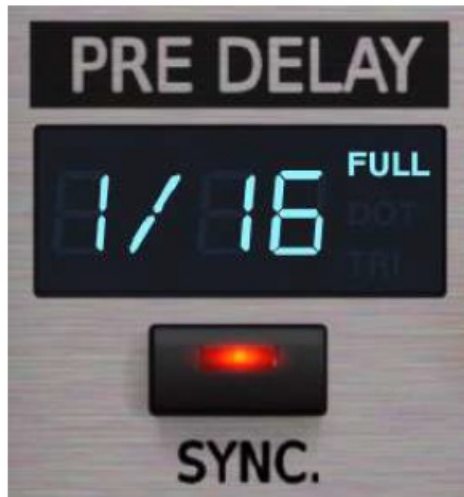
Pre-delay section while Sync. is active
