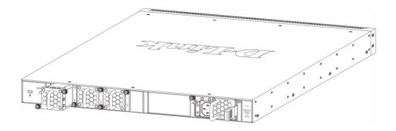
The user can easily remove and insert fan modules into these ports.
