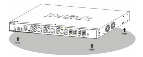
The Switch can be mounted in a standard 19"(1U) rack using the provided mounting brackets. Fasten the mounting brackets to the sides of the Switch using the screws provided.
