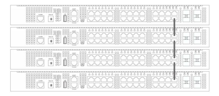
The figure below illustrates how switches can be stacked in a Duplex Chain formation using optical fiber cables connected to SFP+ transceivers or DAC with SFP+ connectors where the 2-port stacking configuration is used.
