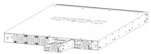
2. Connect the one end of the DC power cord supplied to a DC power module, that will be activated when the AC power is not working, and to a power source (-48VDC/5.2A). Please make sure that connection polarity (positive and negative) is correct.
