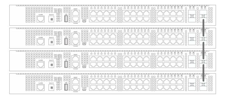
The figure below illustrates how switches can be stacked in a Duplex Ring formation using Category 6a cables with RJ-45 connectors where the 2-port stacking configuration is used.
