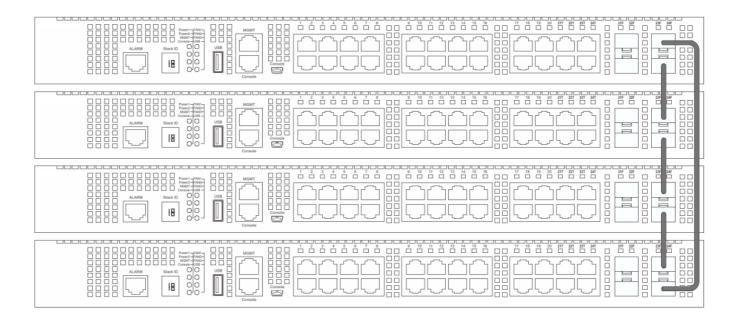
**NOTE:** Stacking Input/Output 1 (SIO1) is a logical stacking port pair. SIO2 is also a logical stacking port pair. A logical stacking port pair must always be connected to the same switch in the stack. Splitting logical stacking port pairs between different Switches in the stack might not guarantee a stable stacking connection.
