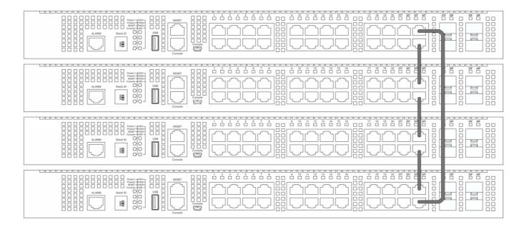
The figure below illustrates how switches can be stacked in a Duplex Ring formation using optical fiber cables connected to SFP+ transceivers or DAC with SFP+ connectors where the 2-port stacking configuration is used.
