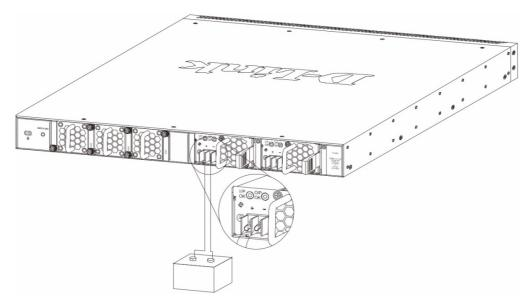
The DC power and AC power of the device will back up each other immediately when one of the power sources fails. If both power sources fail, unplug the switch. When the power source has been restored, plug the switch's power back in.
