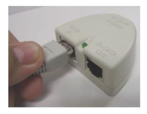
Do Not mistake the "LAN IN" port with the "P + DATA OUT" port. Incorrectly plugging the wrong Ethernet cable into the wrong Ethernet port may cause serious damage to your network devices. D-Link will not replace or repair products or reimburse customers for devices that become damaged due to incorrect installation, nor is liable for any loss of business resulting in the incorrect installation of this product.
