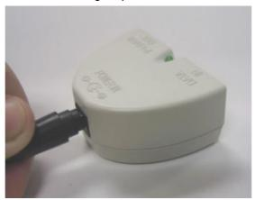
• Connect another Cat 5 Ethernet cable from the Base Unit "P + DATA OUT" to the "LAN IN" of the Terminal Unit.
