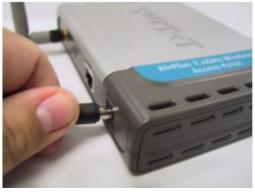
Connect the provided Cat 5 Ethernet cable from the Terminal Unit "LAN OUT" to the RJ-45 LAN port of the Wireless Access Point.
