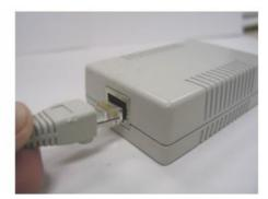
Insert one end of the DC 5V Power Cable that is provided into the Terminal Unit, and the other end into the DC
