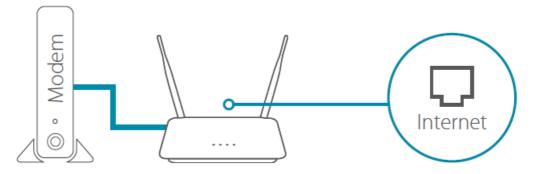
**Note**: If your router does not have a port labeled as INTERNET, plug the Ethernet cable into LAN Port 1.
