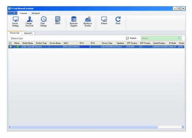
4. Select PC IP address is used to connect the target switch, then click Browse button and select the firmware file (Model name\_ HW ver.\_ FW ver. .hex) on your local hard drive.
