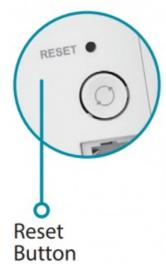
1. If you forgot your Admin password or want to reset your Range Extender back to the factory default settings, press and hold the reset button on the side of the extender using a paper clip and release after the Status light turns red.
