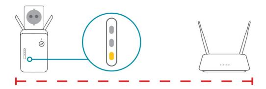
Place the extender in the range of your router. Check the LED indicator on your extender to ensure a proper connection. Green bars indicate a strong signal.
