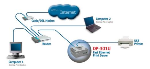
**Warning!** Only a USB printer may be connected to the USB port of the DP-301U. Do not connect any other USB device to the USB port; to do so may damage the unit, voiding the warranty for this product.
