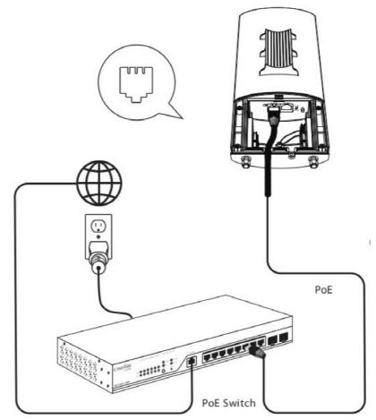
2. Alternatively, you may power the DWL-6720AP by connecting a PoE injector's PoE-OUT (not included into the Package Contents) to the LAN port on the DWL-6720AP. Then connect the PoE injector's LAN-IN port to an available Ethernet port on your switch or router and plug in the injector's power cord into a power outlet as shown below.
