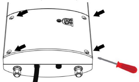
4. Use the grounding wire included into the package contents to ground the access point.
