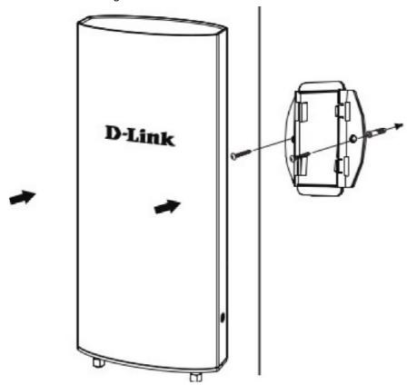
6. Attach the access point to the wall.
