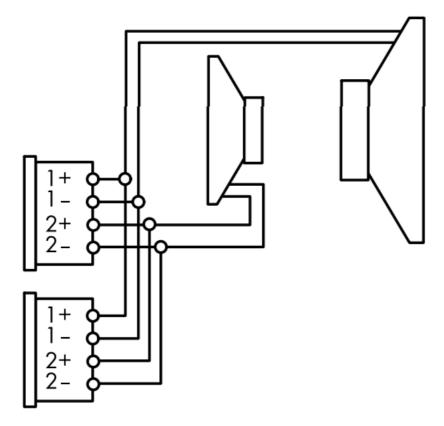
**NLT4 F/M Connector wiring**
