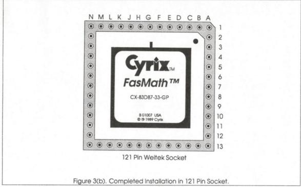
6. Examine package from all sides to be sure all pins are going in correctly. If there are any bent pins, remove the CX-83D87 and straighten the pins before going on.
