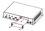
3. Gently pull the card straight out of the module slot, using the provided handles.
