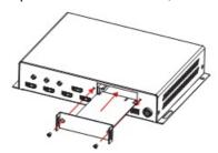
3. Align the card with the guide rails to each side of the module slot, and gently slide the module card into the slot until its faceplate is flush with the back of the unit.
