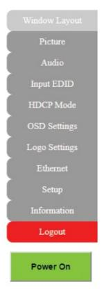
• Clicking the red "Logout" tab will automatically log the currently connected user out of the WebGUI and return to login page. Clicking on the "Power" button will toggle the unit's current power state between on (green) and stand-by (red).
