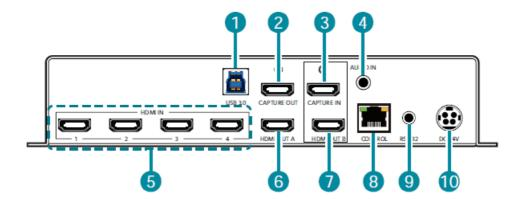
USB 3.0 Port: Connect directly to a PC's USB 3.0 port to control and power the video capture component of the unit.
