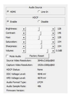
1. **Audio Source:** Switch the audio source to record between the embedded HDMI audio and the analog line input.
