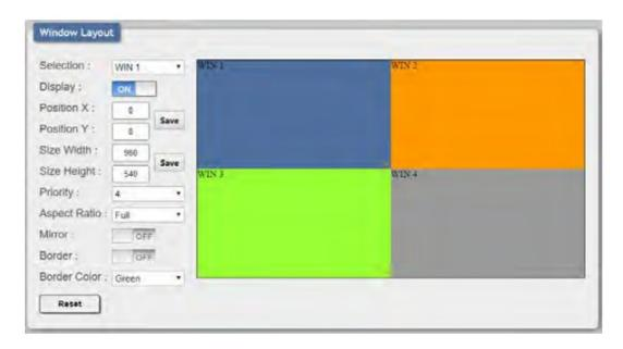
1. **Selection:** In multi-windowing modes, use the dropdown to select the window to modify. In Matrix mode select the input to modify.
