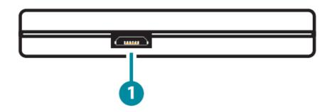
1. **USB Port:** Plug a 5V Micro-USB power supply into this port to inject additional 5V power into the HDMI signal. (Optional)
