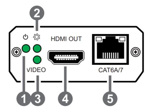
1. Power ( ) LED: This LED will illuminate to indicate the unit is on and receiving power.
