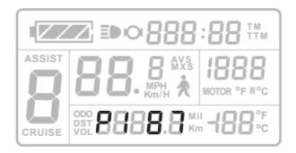
Range 1-255. XF800 default code is 87; When you see P1 is flashing, press or to change data required. This technical setting is only for engineer setting, do not modify or change the setting
