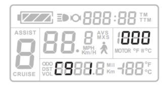
Range: 0-1, XF800 default code is 0; 0—Inactive LCD restart password function; 1– active LCD restart password
