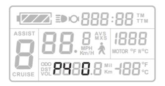
Range: 0-1, 0 means zero boost; 1 means non zero boost. XF800 default code is 0; In the zero boost also called hard boost which means, once you use the throttle or pedal assistant, you get will push from the motor immediately; In non-zero boost, you have to use pedal first to move the e-bike to some certain speed and the
