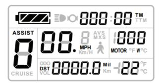
Press for seconds to turn or turn off the bike computer; if the motor stops for over 5 minutes without any movement and the bike computer will automatically shut down.
