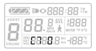
Range: 0-1 XF800 default code is 0; 0-Inactive cruise control function, 1-active cruise control function; Press switch to C7, press or to change data required.
