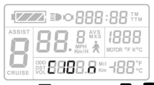
Range: n/y, XF800 default code is n, Press switch to C10, press or to change data required. n— inactive or no y—active or yes,
