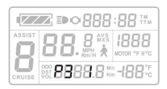
Range: 0-1; XF800 default code is 1; 0-Speed Control Mode; 1- Copying Torque Control Mode; Press switch to P3, press or to change data required. This technical setting is only for engineer setting, do not modify or change the setting.
