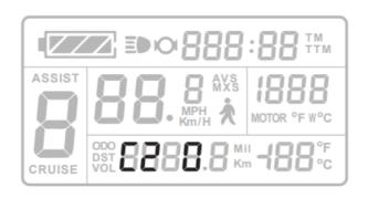
Range: 0-7, XF800 default code is 0; Press switch to C2, press or to change data required. This technical setting is only for engineer setting, do not modify or change the setting.
