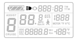
After turning on the computer and press for 3 seconds to turn on or turn off the front light.
