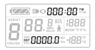
Press + together for 2 seconds after turning on bike computer over 5 seconds. When you see LCD image-TM and DST are flashing as below and press to clear the TM and DST data.
