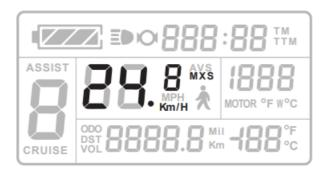
Range: 1-72KM XF800 default setting code is 72KM (which means no limit on speed) Press + together for 2 seconds after turning on bike computer within 5 seconds. When see the max speed is flashing as image below and press • or • to change the Max speed setting, and the default Max speed for XF800 is
