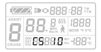
Range:0-10, XF800 default code is 10; Press switch to C5, press or to change data required. Those technical setting are only for engineer setting, do not modify or change the setting.
