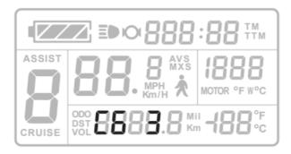
Range:1-5, XF800 default code is 10; 1 means the darkest and 5 means the brightest. Press switch to C6, press or to change data required.
