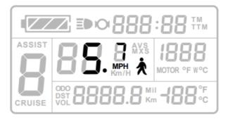
After turning on the bike computer and pressing for 3 seconds to activate the walk mode, release the button, and walk mode will be automatically canceled.
