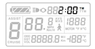
After turning on the bike computer and press one time to switch and check data of AVS/MAX/TM/TTM/DST/ODO/VOL
