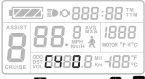
Range:0-4; XF800 default code is 0; Press switch to C4, press or to change data required.
