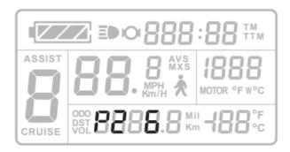
Rage:0-16, XF800 default code is 1; Press switch to P2, press or to change data required. This technical setting is only for engineer setting, do not modify or change the setting
