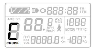
Riding at a speed above 7 km/h, hold the for 3 seconds to activate cruise control. Use the break to cancel the cruise control.
