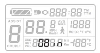
Range is 6-28 inch and 700C. XF800 default rim setting is 26 in. After setting Max Speed, press to switch wheel rim diameter setting. When you see the rim data is flashing, press or to change the data of rim diameter.
