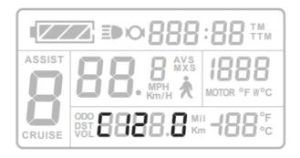
Range:0-7, XF800 default code is 4. This technical setting is only for engineer setting, do not modify or change the setting.
