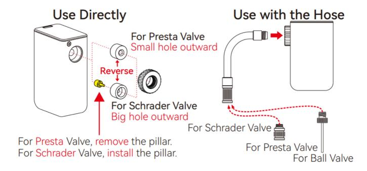
The inflator is ready for the Presta valve right out of the box. For the Schrader valve, please adjust the nozzle accordingly. The hose can be directly connected and used, regardless of the presence of a pillar in the nozzle. When the target air pressure is above 100 PSI, please use with the hose to prevent air leakage from the nozzle.
