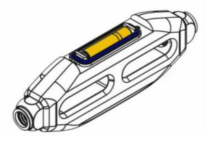
Check the 'O' ring seal (shown in blue) is seated properly and re-lubricate if dry.
