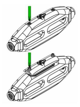
Lift off the plastic battery cover and place down without disturbing the seal on the body.
