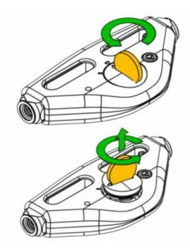
Replace the CR2032 battery with equivalent. Do not use non-standard batteries or other sizes, as this can cause damage.
