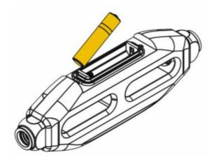
Remove the old batteries and replace with 2x new AAA.
