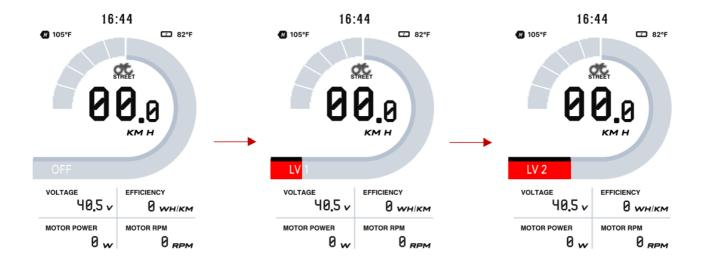
There are 3 sets of assist levels; 3, 5 & 9. To change the assist levels set, long press the MENU button upon within 15 seconds upon startup and access ALL GEAR in the main settings page.
