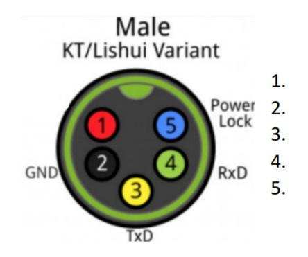
1. Red wire: Anode(36V to 72V)
