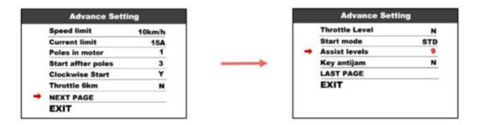
The power output will be distributed evenly across the chosen number of assist levels (or gears) according to the Assist Level Configuration and Speed Limit Assist settings on your CYC Motor (BAC) mobile app:
