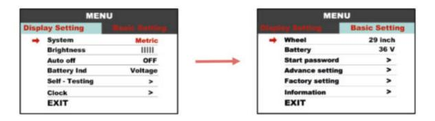
Press the UP/DOWN buttons to change between the parameters, the MENU button to select, & UP/DOWN to change the selected parameter.
