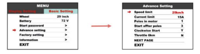
Go to the NEXT PAGE on the display. Here, you can choose the number of assist levels (or gears) accordingly. The available options are 3, 5, or 9 assist levels.
