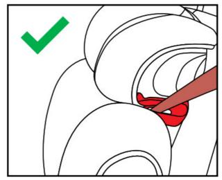
**WARNING!** The diagonal belt must run back at a recline and must never run forward to the upper belt point in your vehicle. If it is not possible to adjust the seat in this way, e.g. by pushing the child seat forward or using it on another seat, this child seat is not suitable for your vehicle.
