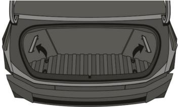
Use a 10mm socket to remove the exposed bolts (4x). Install the L-track brackets (B & C) using the same bolts.
