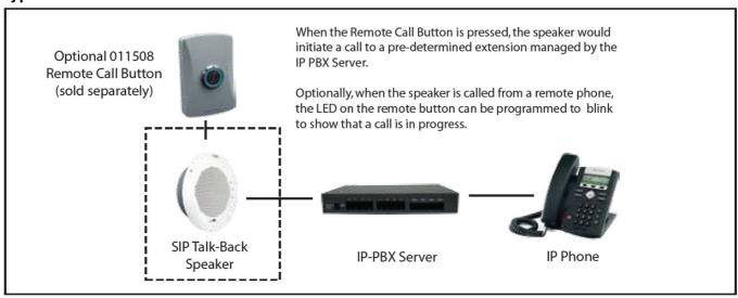
When the Remote Call Button is pressed, the speaker would initiate a call to a pre-determined extension managed by the IP PBX Server.
