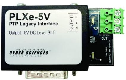
The Cyber Sciences Precision Timing Protocol (PTP) Legacy Interface (PLXe-5V) is a wiring adapter for the CyTime™ Sequence of Events Recorder to output a legacy time protocol to other devices. The adapter fits the "Options" port (DB15 connector) of the SER-32e and facilitates wiring of 5V signals via a screw-type terminal, suitable for power equipment wiring.
