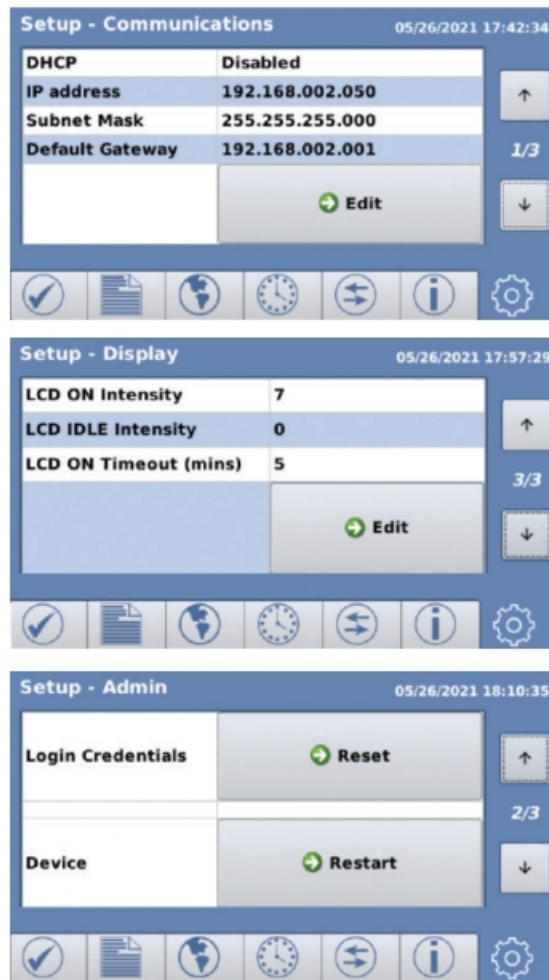
Figure 4-3. Initial setup via LCD/keypad
