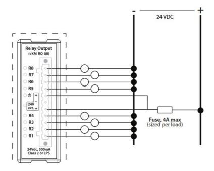
18 AWG (Belden 8760) shielded twisted pair cable is recommended for all input and output connections.
