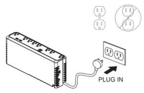
3. Plug the UPS into a 2-pole, 3-wire ground-ed receptacle (wall outlet). Make sure the wall branch outlet is protected by a fuse or circuit breaker and does not service equip-ment with large electrical demands (e.g. air
