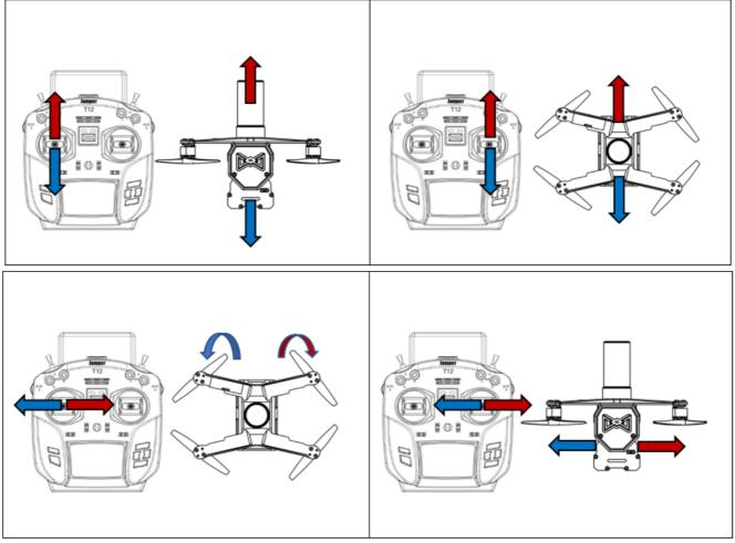
3. After landing, stop the propellers by moving the left throttle to the left and down, and hold it in this position until the propellers stop.
